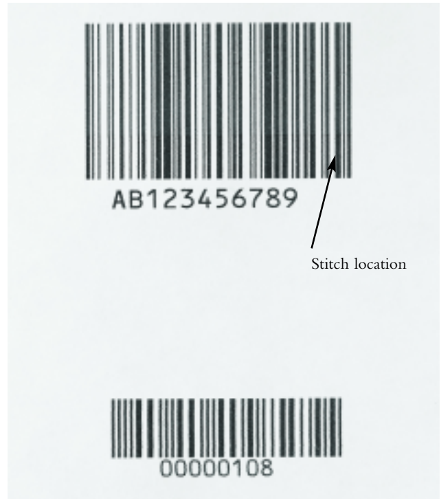
122mm (4.8") print swathe printed at 421 x 316dpi including electronic image stitching with two print heads
